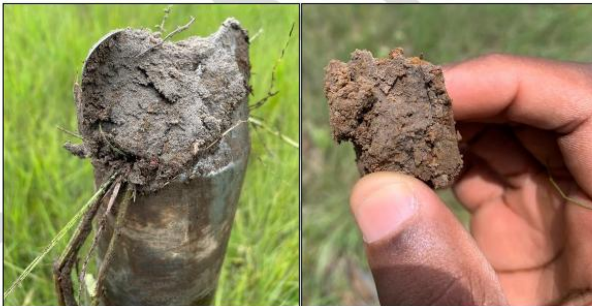
Figure 4-14: Representative photographs of soil samples within dambo wetland systems, illustrating typical soil morphological characteristics including mottling (right) and gleying (left) associated with a fluctuating water table
